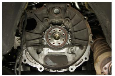
3. Remove factory release components. Clean transmission again. Do not damage the input shaft seal.
