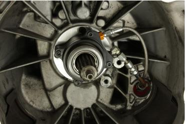
6. Using the supplied P-clamp, mount the hydraulic lines to the factory slave cylinder mounting bolt location. Tighten bolt to 8ftlbs.
